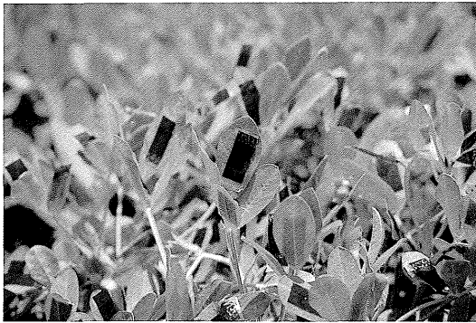
Fig. 1. The upper leaves of the canopy with the integrated solarimeter films in the control of the 40 cm spacing around noon.
