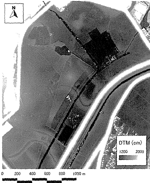
Fig. 3. DTM developed by using the minimum values from the two DSMs acquired after the controlled burns (April 2006 and 2007).
