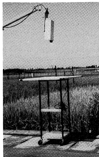
Fig. 4. The portable spectrophotometer measuring the reference panel (1 m × 1 m).
