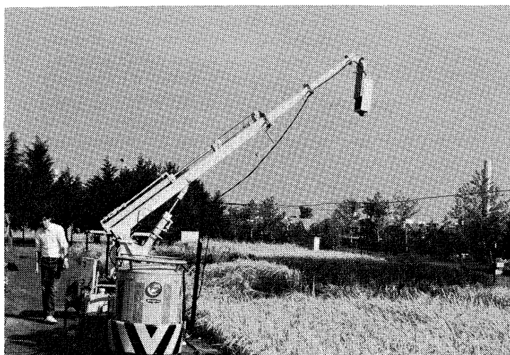
Fig. 3. The motorized crane and the photometer used to obtain the spectral signatures from paddy rice canopies.
