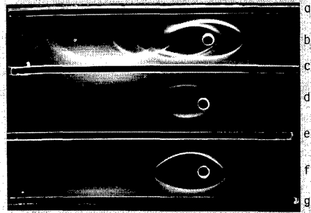
Fig. 4. Immunoelectrophoresis of the purified LIgG. Ten \mu\text{l} of sample was applied to a well and electrophoresed at a constant voltage of 6 v/cm. a, e (basins), anti-LIgG. b (well), mouse normal serum. c (basin), anti-mouse whole serum. d (well), purified LIgG. f (well), IgG from CA12 ascites fluid. g (basin), anti-mouse IgG.
