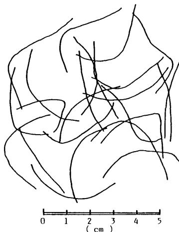
Fig. 5 The sample of curved lines that is used for the length measurement. The real length of sample is 100 cm.
