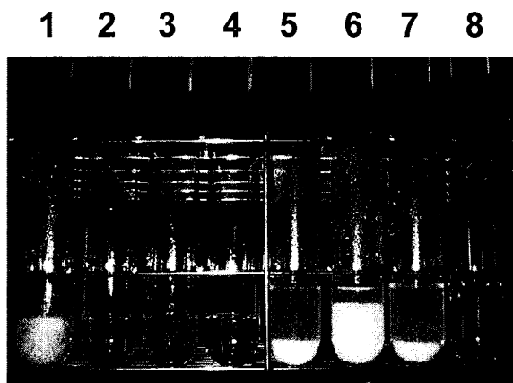
Fig. 2. Precipitation of enzymatically hydrolyzed guar gum (EHGG) in the alcohol precipitation method
