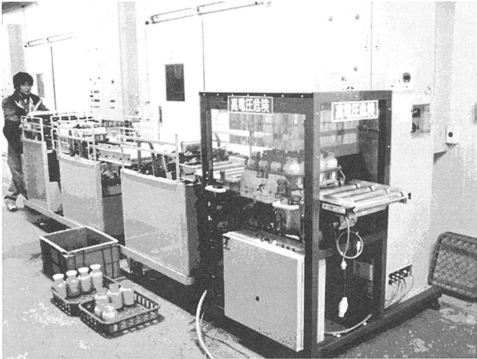
Fig. 1 Inline setting of the electric impulse installation.
