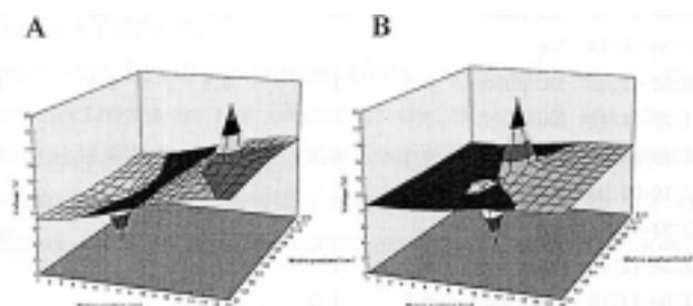
**Fig. 2.** The model of intensity slope of the electric field around the electrodes measured by field mapping methods. A: Electric Field Experiment (0.675 A, 60 Hz, 34 per mil) ; B: Partial Electric Field Experiment (1.03 A, 60 Hz, 34 per mil).
