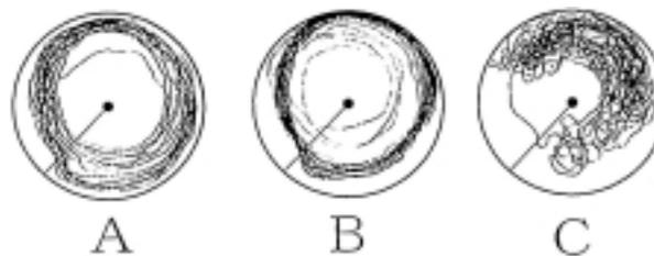
**Fig. 5.** The tracks of the swimming patterns of the silky shark, *Carcharhinus falciformis*. A: no stimulation (normal); B: 60 Hz sine wave electric field; C: DC pulse electric field.
