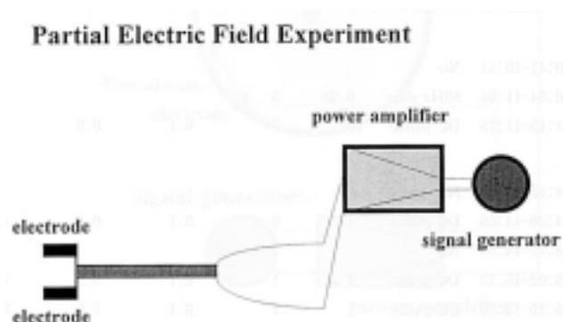
**Fig. 3.** Outline of the methods for the Partial Electric Field Experiment (PEF).
